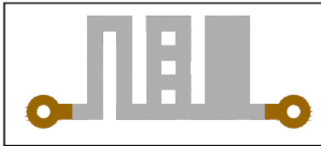
▲ Trimnable resistor Ladder network
