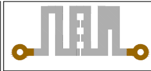
▲ Trimmed multiple square resistor
